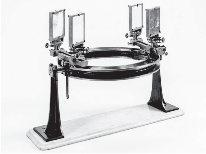
Fig. 4: Original interferometer constructed by Ludwig Mach, ca. 1892
